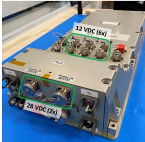
Figure 5.1.6-1: 12 and 28 VDC Power Interfaces on PIU2
