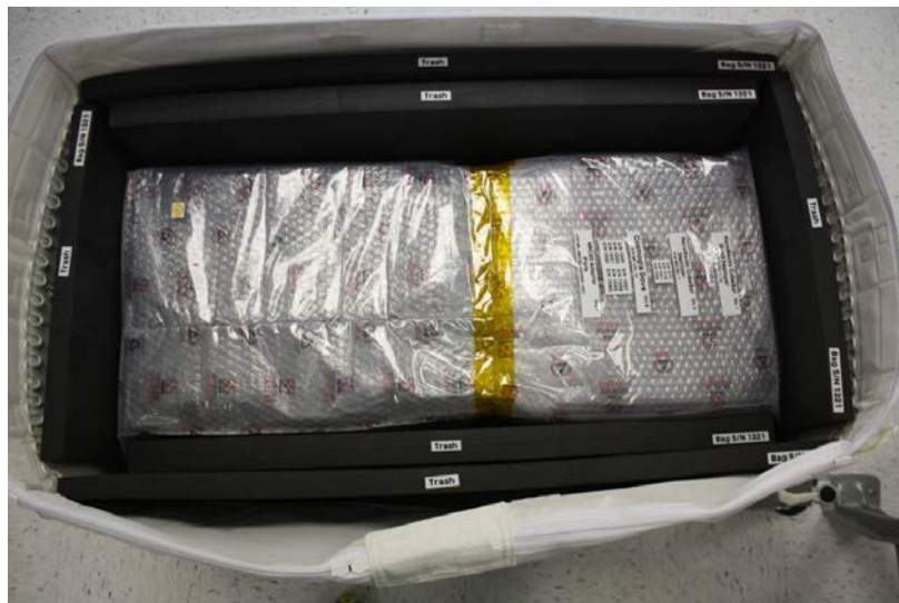
Figure 3.4-1: Sample NRCSD Stowage Configuration for Launch (NRCSD Quad-Pack in M2 CTB)
