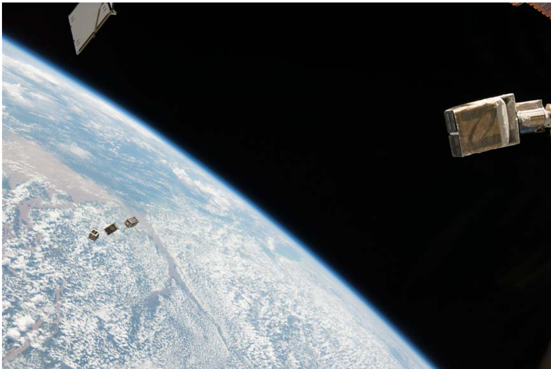
Figure 3.4.3.4-3: NRCSD Deployment of Three (3) CubeSats from ISS (Photo Credit: NASA)
